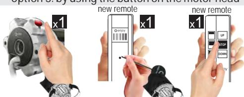
1. Press 1 time on the button from the motor head
