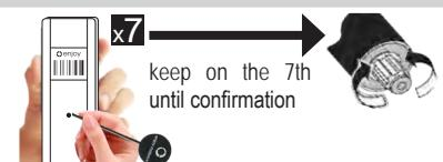
1. Press 7 times on the programming button P3, at short intervals, holding down the 7th time for ± 4 seconds
